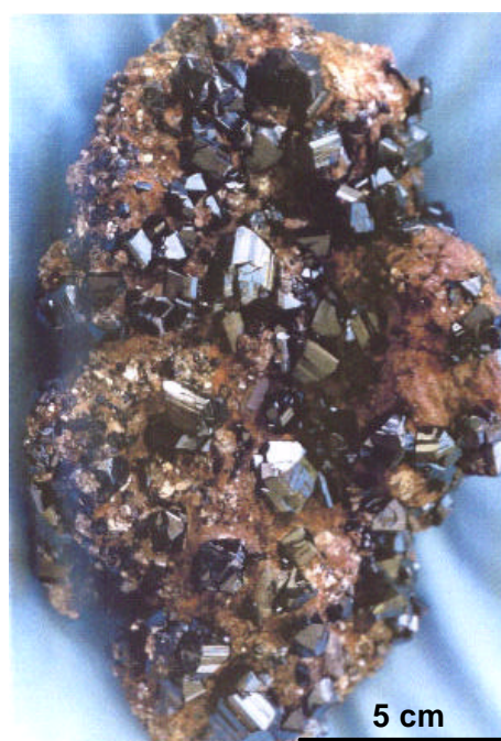
Figure 2: A spectacular specimen of tin-bearing greisen collected from Sheep Station Hill 30 years ago. Large cassiterite crystals are shown clustered within very micaceous greisen. (Photograph courtesy of Mr Bob Smith.)
