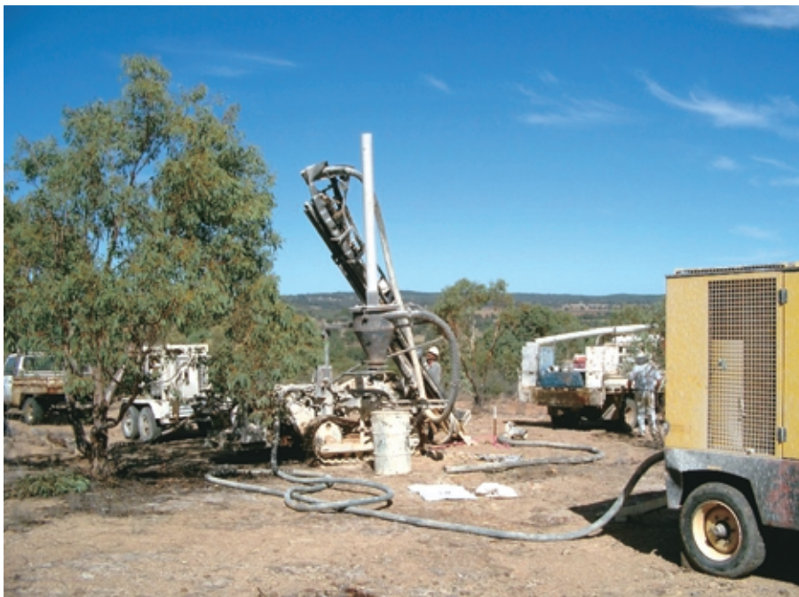
RC drilling at the Elsmore tin project in northern New South Wales.
