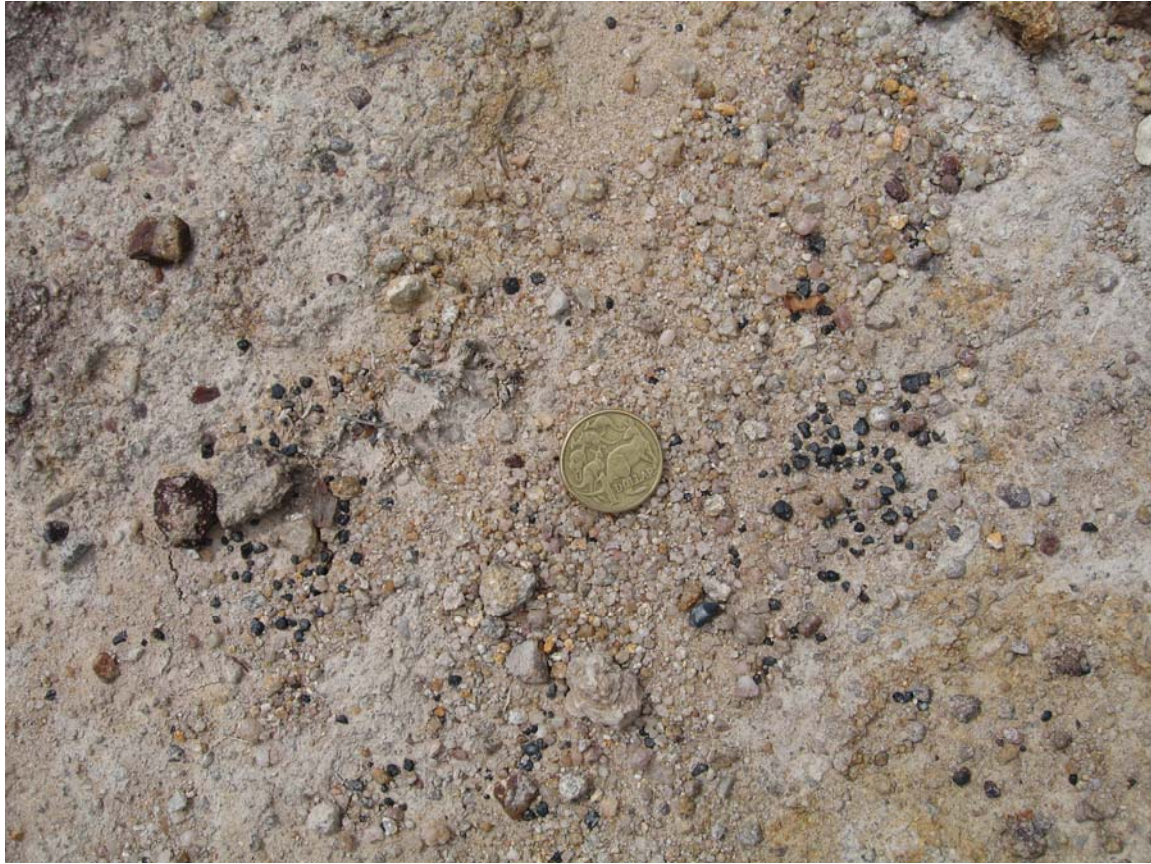
FIGURE 3: Semi-consolidated alluvium at Newstead with abundant tin occurring as free grains of cassiterite (black grains in photos).
