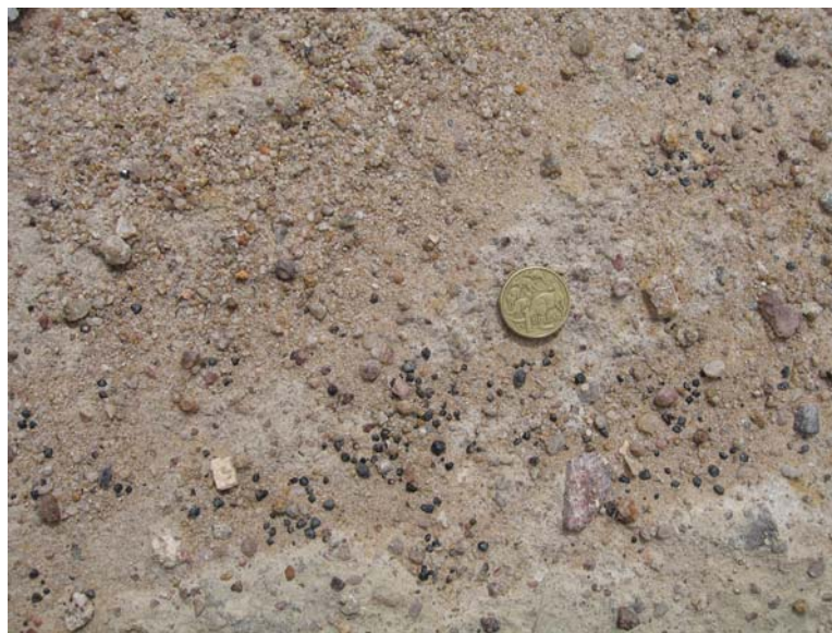
Figure 5: Coarser grained variant of the Karaula Lead, with cassiterite (black grains) on surface
