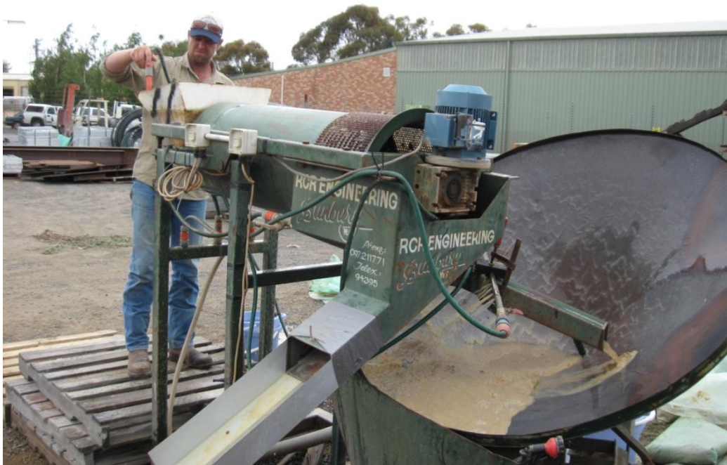
Figure 4: The cone concentrator to be used by Malachite to test the Karaula Lead bulk samples for recoverable tin
