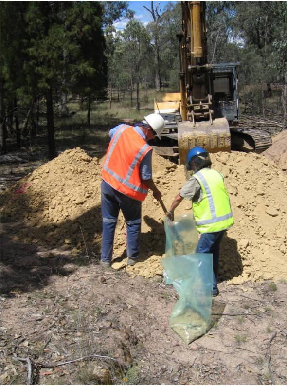
Figure 2: Collecting bulk samples of the Karaula Lead to test for recoverable tin
